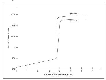
Figure 15-4 First Stage Cyanide Oxidation - Typical Titration Curve
